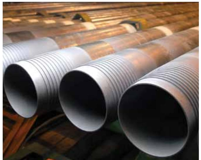
▲ Dopeless® technology is a fully engineered solution, applied at the mill in a completely controlled industrial process.
